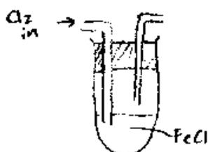
Example 4 – Appropriate apparatus set up for Reaction B (although there is a missing outlet tube through the left hole of the stopper.)
