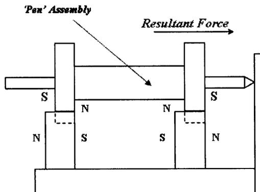
**Figure 2 Simplified diagram of one possible working principle of the Floating Pen.**
