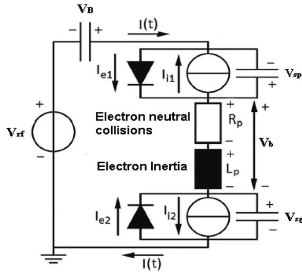
FIG. 2. Schematic diagram of the electrical circuit equivalent to the CCP discharges. Here  $I(t)$  represents the rf current,  $I_{e1}$  and  $I_{i1}$  represents the electron and ion current to the powered electrode sheath, and  $I_{e2}$  and  $I_{i2}$  represents the electron and ion current to the grounded electrode sheath.
