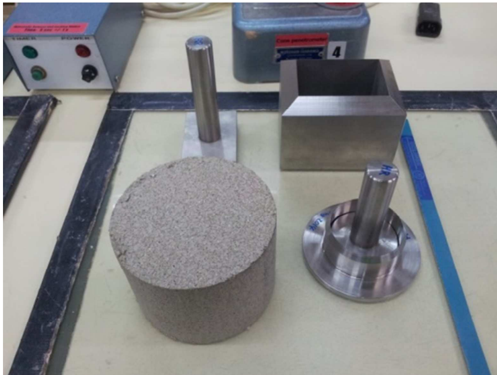
Figure 2. Initial block of sample and cutters used for preparing VL specimens 381x285mm (96 x 96 DPI)
