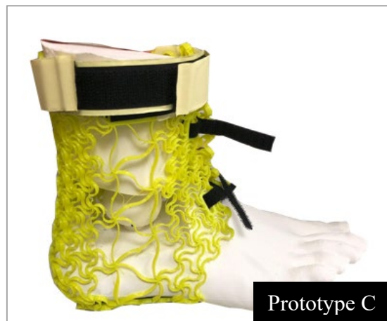
310 Figure 10: Ankle brace prototype A (diamond mesh design), prototype B (oriental design) 311 and prototype C (“horseshoe” design)
