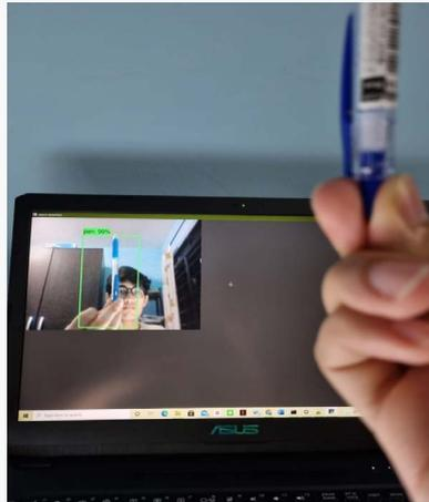
As for objects such as the pen (Figure 7), the Object Detection model has its limits because it is not able to identify and distinguish a pen and a pencil clearly even after training sufficient images of these two objects. This is due to the resemblance of the two objects in terms of the size and shape. Hence, it is necessary to avoid training images of these types of objects so as to maintain accuracy and consistency of the model.
