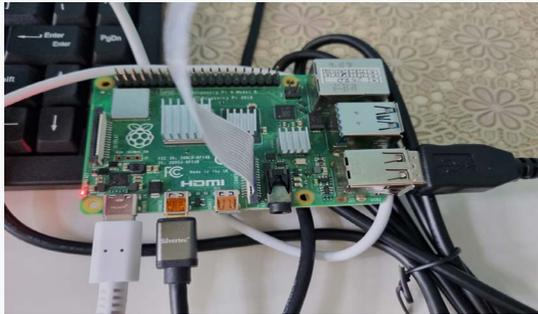
With reference to Figure 4, the Raspberry Pi serves as the CPU of a desktop. The Raspberry Pi is able to work as a mini version of a CPU and hence is able to keep the device at a small form factor in order to be user-friendly for kindergarteners.
