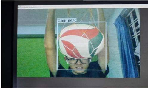
As for the coin (Figure 8), the Object Detection model's accuracy and consistency started to decline as the camera focused on objects that are circular or spherical. The model will persist in detecting the coin as other types of round objects such as a ball as seen in Figure 9 and vice versa. It is quite seldom that the model will detect the coin correctly at high accuracy and consistency as shown in Figure 8.
