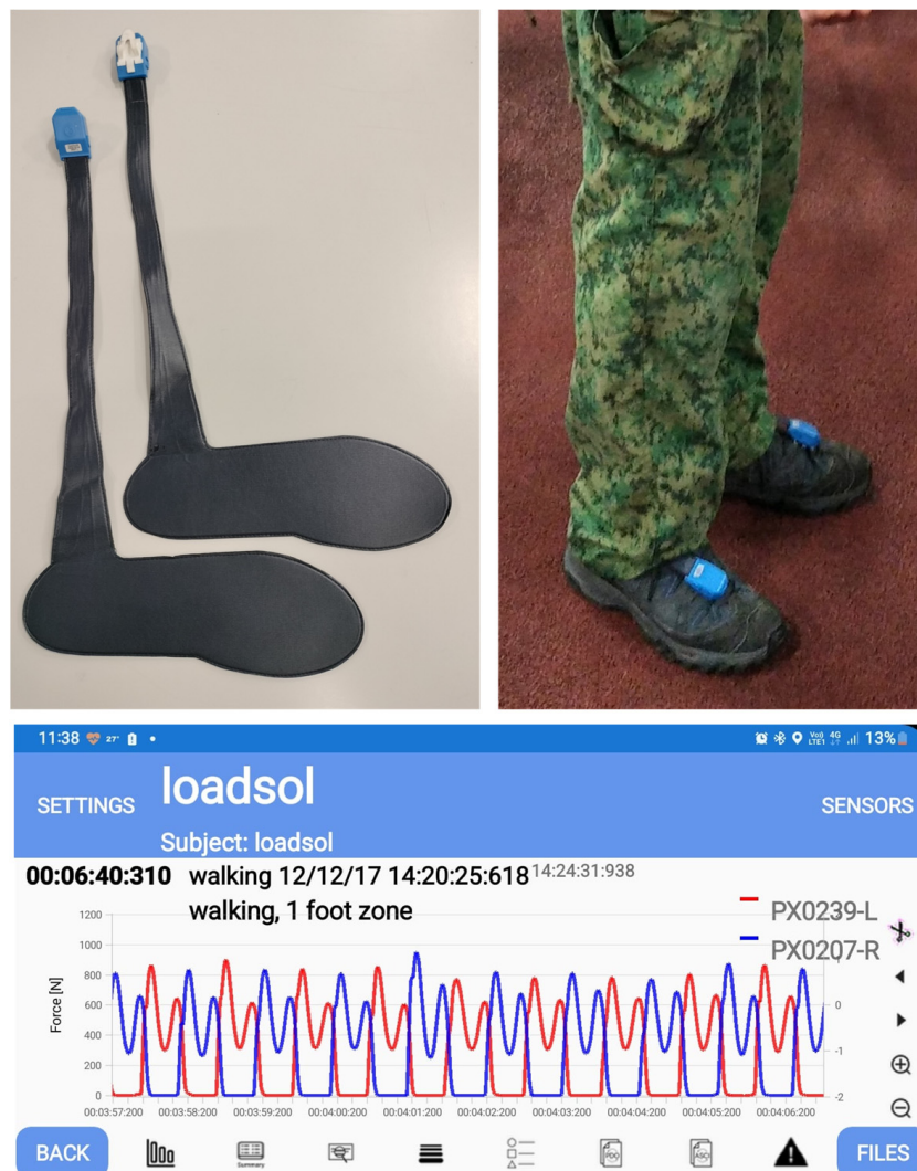
Figure 1. The loadsol ® wireless in-shoe sensors were fitted into participants' military boots to measure normal ground reaction forces during walking via the loadsol-s mobile phone app (version 1.7.51).
