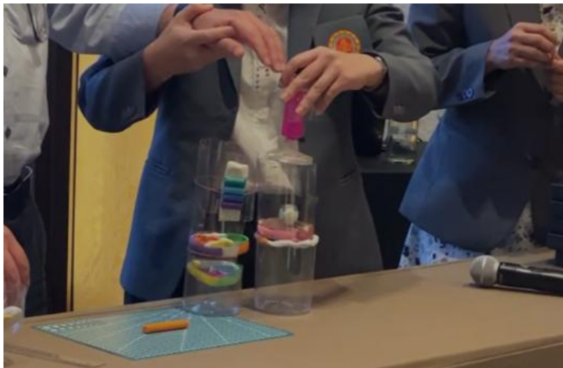
Figure 4. Group 3 prototype was a push cutter. The clay was used to make the sieves. However, these were not secure and hence, the sieve was pushed down together with the plunger. The concept on how the prototype worked, however, was communicated.
